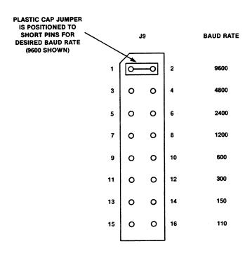
FIGURE 2-12. Host Baud Rate Select Jumper (J9)
