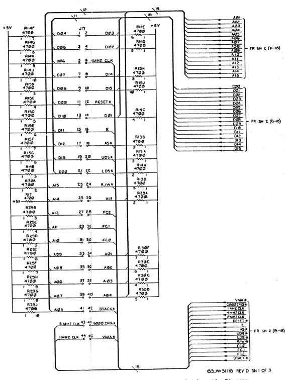
FIGURE 8-3. MEX68KECB MC68000 Educational Computer Board Schematic Diagram (Sheet 1 of 3) 8-13/8-14
