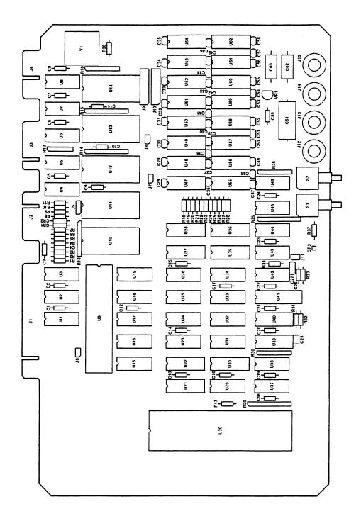
FIGURE 8-2. MEX68KECB Parts Location Diagram
