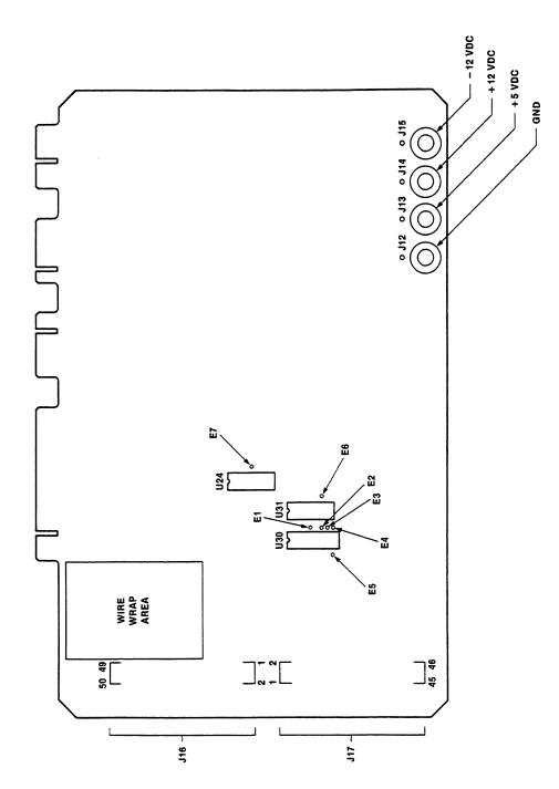
FIGURE 7-2. MEX68KECB Signal Connection Points For Wire-Wrap
