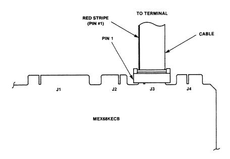
FIGURE 2-8. Terminal Cable Connection to MEX68KECB
