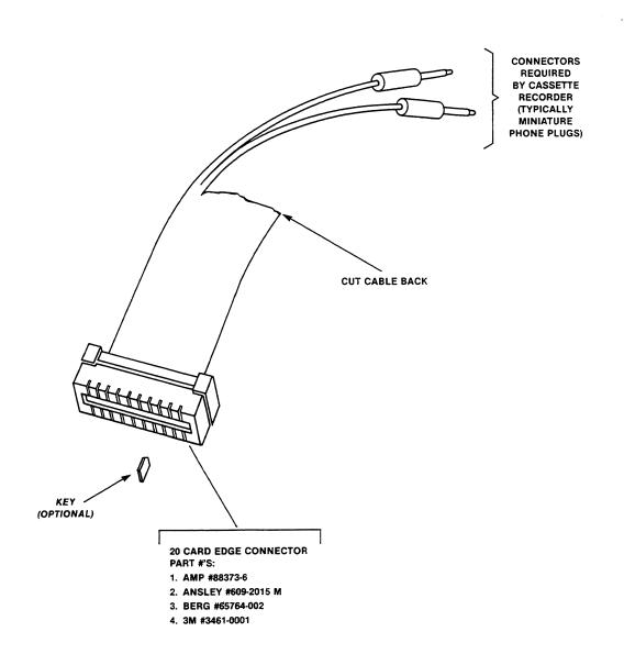
FIGURE 2-15B. Cassette Recorder Cable Detail
