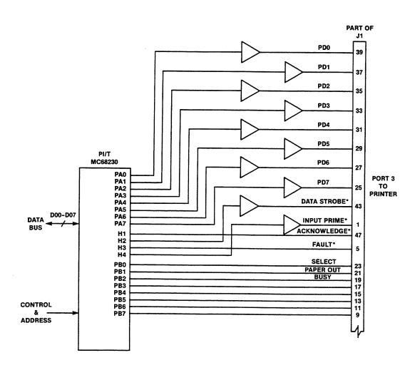
FIGURE 6-5. Printer Interface Port 3 Functional Schematic Diagram
