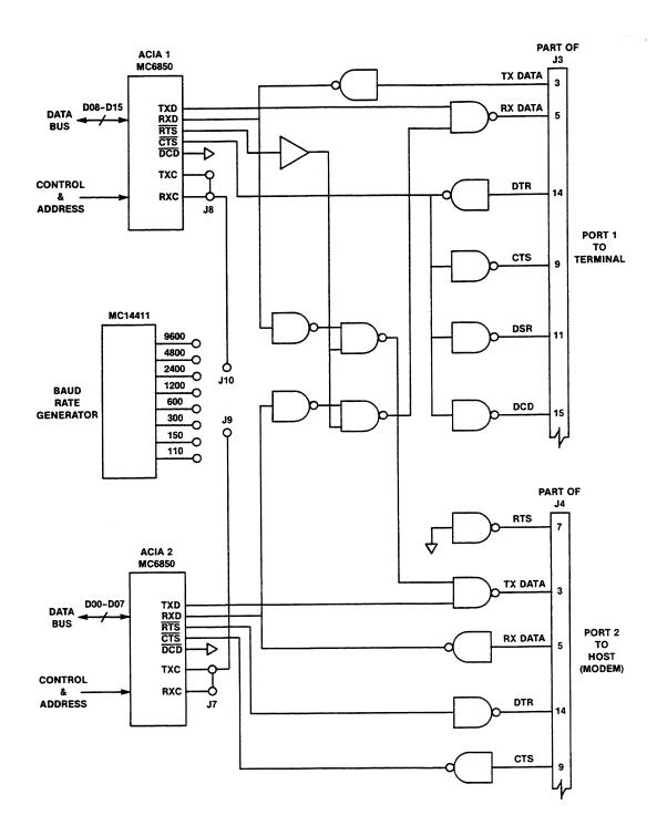
FIGURE 6-4. Serial Communications Ports Functional Schematic Diagram
