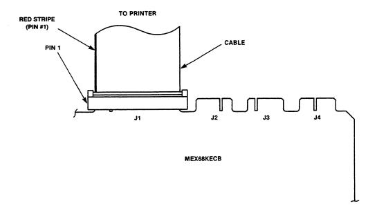
FIGURE 2-11. Printer Cable Connection to MEX68KECB
