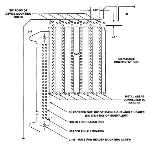
NOTE: METAL AREAS CONNECTED TO +5.0 VDC ON OPPOSITE SIDE OF BOARD
