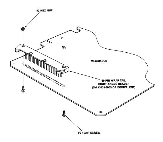
FIGURE 7-4. Auxiliary I/O Header Mounting Detail
