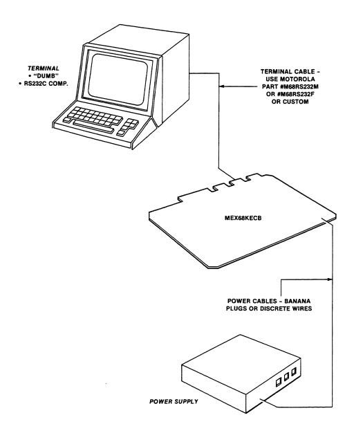
FIGURE 2-6. Minimum System Configuration
