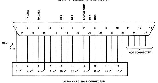
FIGURE 2-7. Terminal Cable Detail and Signal Line Connections
