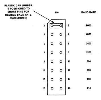
FIGURE 2-5. Terminal Baud Rate Select Jumper (J10)
