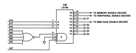
FIGURE 7-5. Address Decode Logic For Memory Map Primary Segments
