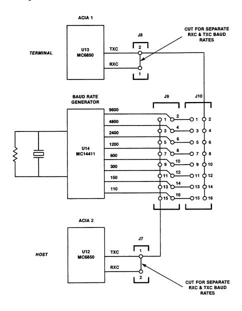
FIGURE 2-4. Interconnection Diagram for Baud Rate Selection
