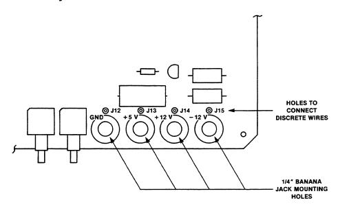
FIGURE 2-3. Detail Showing Location of Holes J12, J13, J14, J15 to Connect Discrete Power Wires
