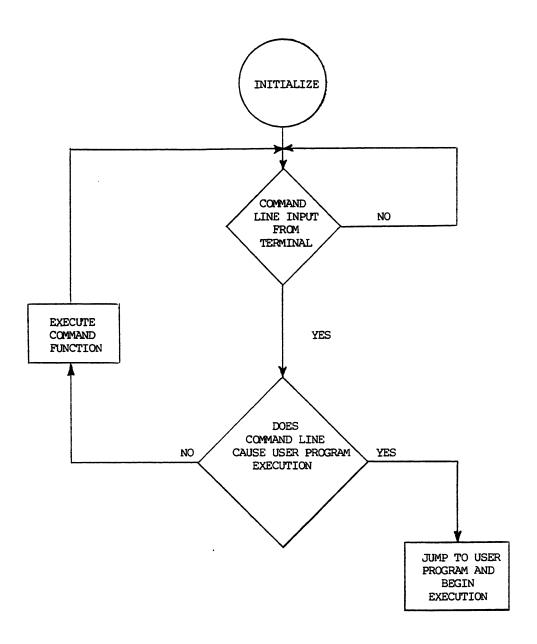
FIGURE 3-1. Flow Diagram of TUTOR Operational Mode
