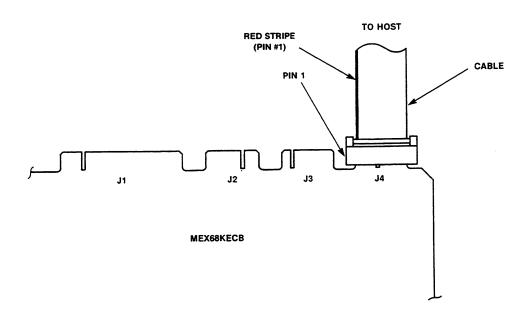
FIGURE 2-14. Host Computer Cable Connection to MEX68KECB
