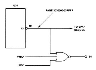
FIGURE 7-7. M6800 Page Address Signal Generation
