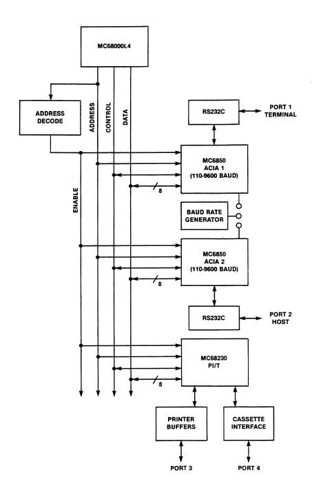
FIGURE 6-1. System I/O Block Diagram
